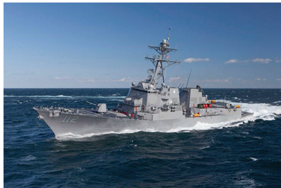
Figure 3. U.S. Navy guided missile destroyer DDG112 Michael Murphy cost $1 billion, is 155 meters long, displaces nine thousand tons, is crewed by about 320, and is equipped and trained to simultaneously engage in a variety of missions.
